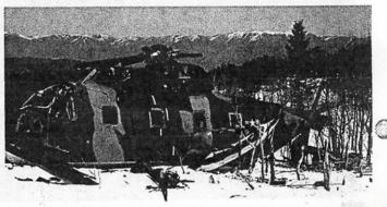
The main rotor blade sheared the tail boom and ripped into the cockpit
