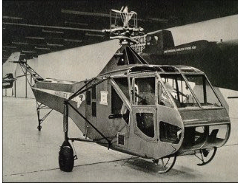
The Sikorsky VS-316A (military designation R-4) was a definitive development of Igor Sikorsky's successful pre-war VS-300, and in 1944 became the first helicopter in the world to be placed in series production.
