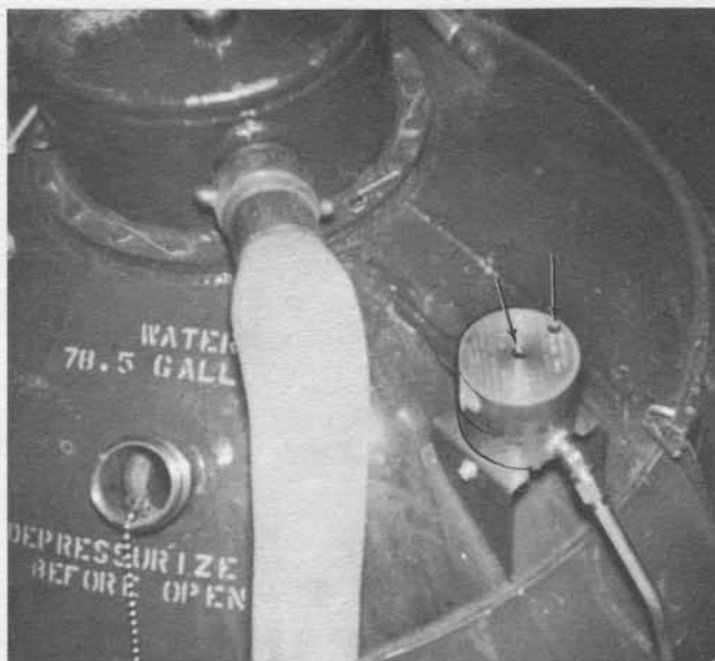
CRITICAL ADJUSTMENT of these hex set screws must be done in base shops to avoid possible malfunction at the scene of an incident.
