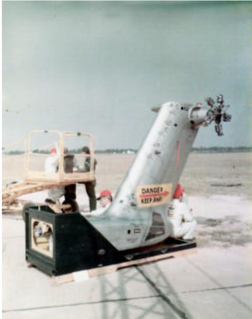
The pylons are mounted in the jig with its mounting bolts and marked with the aircraft tail number.
