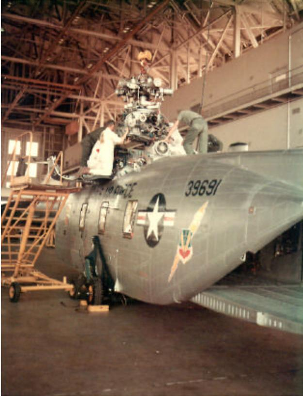
Sikorsky's first attempt to load the helicopter was made with the engines and doghouse cowl installed and there wasn't enough overhead clearance. After these items were removed the second try went fine. The first fuselage was moved to the C-133 front bulkhead using the aircraft interior winch, hooked to front gear. Blades were stored inside the fuselage. Transmissions were stored behind first helicopter
