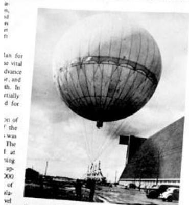
Figure 24. This inflated balloon shows the geometry of the many paper gores which make up the gas-proof envelope. Nineteen shroud lines attached to the cloth skirt carry the gondola. (U.S. Navy photograph, 80-G-326353, in the National Archives)
